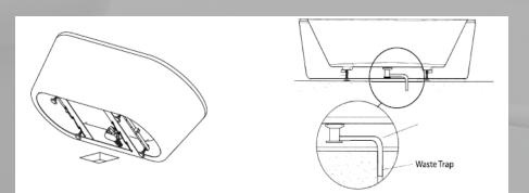
To test for any leaks pour some water in the bath, open the pop up waste and make sure all the water runs into your buildings grey water system
