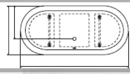
Drill a hole in the floor for the draining pipe
